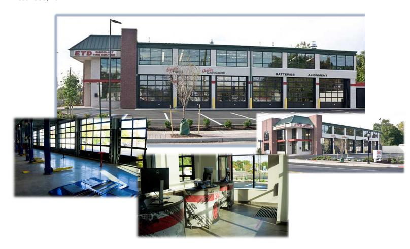
ETD Westwood is a ground-up, 8,445 ft² service center. The construction featured use of a pre-engineered steel building with a standing seam roof. The façade also used decorative split face block walls. The interior contains six service bays with sectional glass doors, recessed alignment racks, customer service, waiting area, restrooms. The construction also included second floor tire and parts storage. Site improvements included drainage, curbs, sidewalks, paving, lighting, and landscaping.
